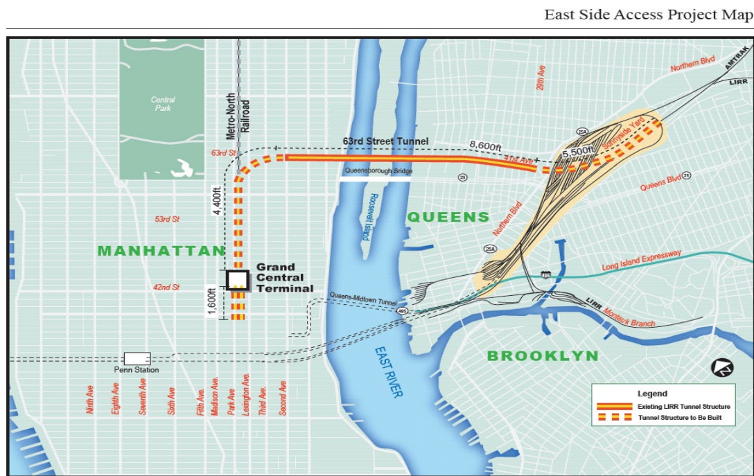
MTA/LIRR East Side Access Project
