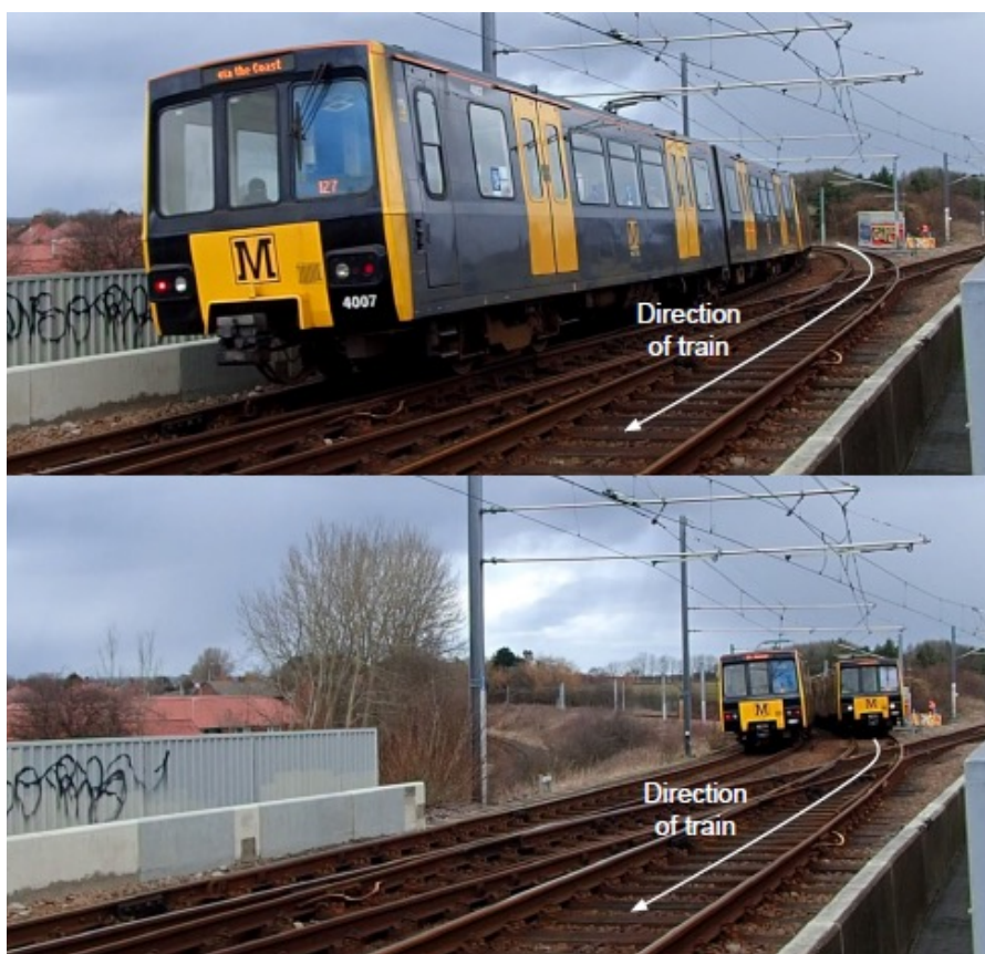
Figure 4-3 Outbound train on far track obscures vision of inbound train near track at work location 19
