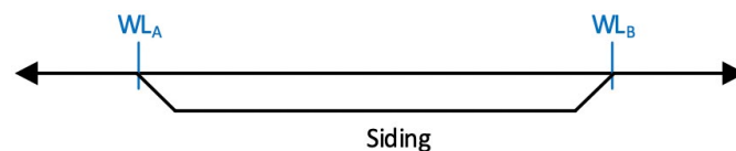
Figure C-6 Single track with siding
