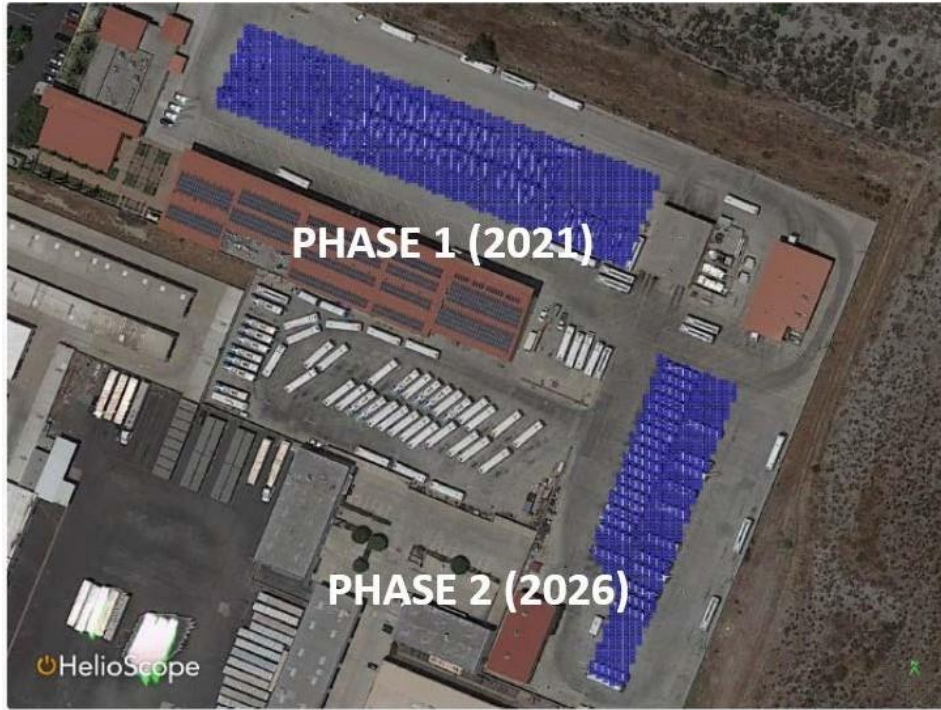
Figure 5: Arcadia Depot Solar Layout
