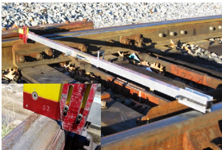
Figure 7-3 Switch inspection gauges built by NS
