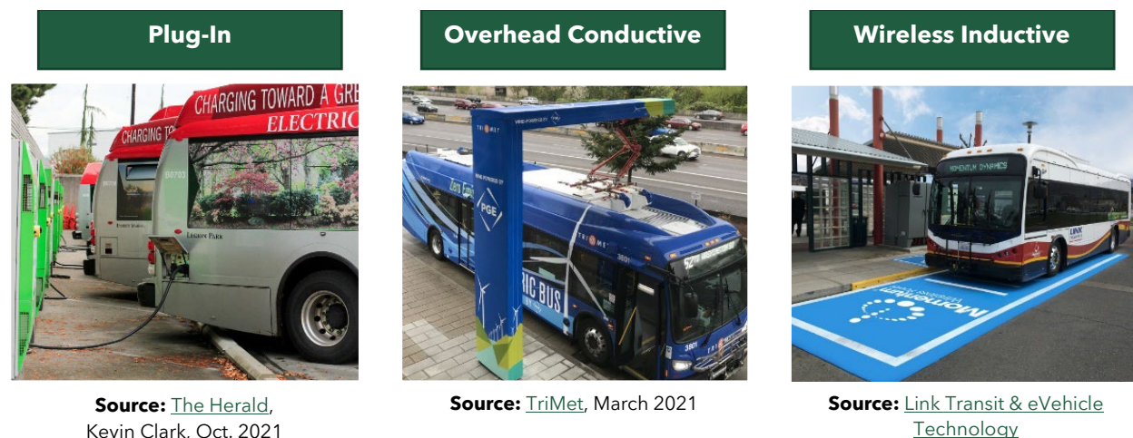
Figure 5: BEB Charging Infrastructure
