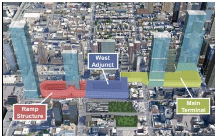
Rendering showing the main components of the PABT Replacement Project. Image source: Port Authority of New York and New Jersey
