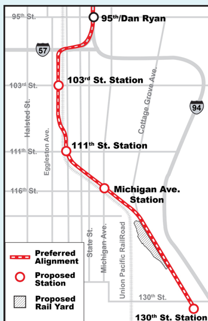
Figure 8 – Map of proposed new Red Line Extension. New stations proposed at Michigan Avenue and 130th Street are anticipated to have off-street facilities for bus connections that could potentially also serve as on-route electric charging locations.
