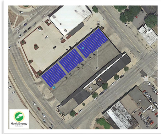
Aerial site plan of the Transit Center canopy roof showing where the solar panels will be placed
