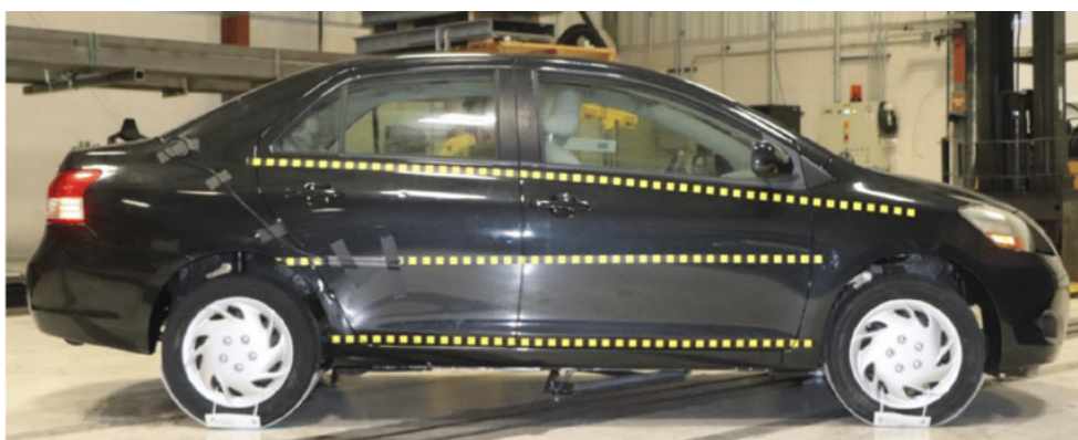
Figure 5-45 Location of Inch Tape on the 2010 Toyota Yaris (pre-test)
