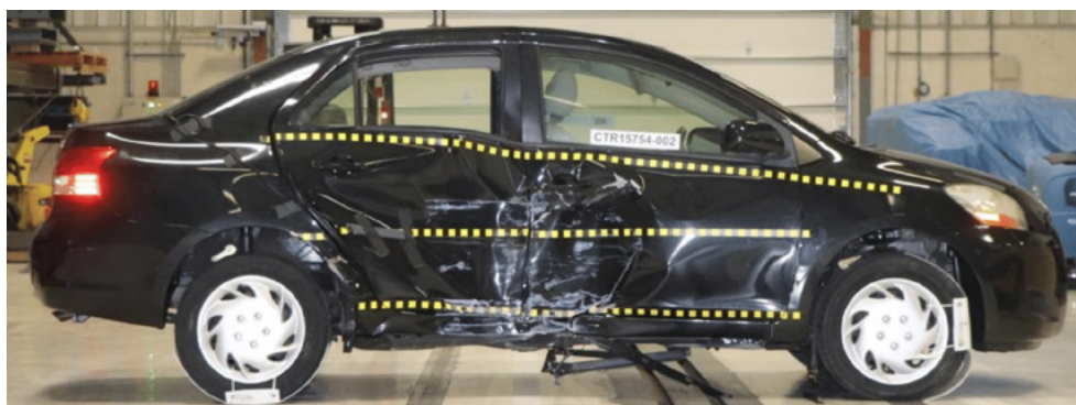
Figure 5-46 Impact Damage to the Yaris in Test 2 Where Inch Tape Measurements Were Made
