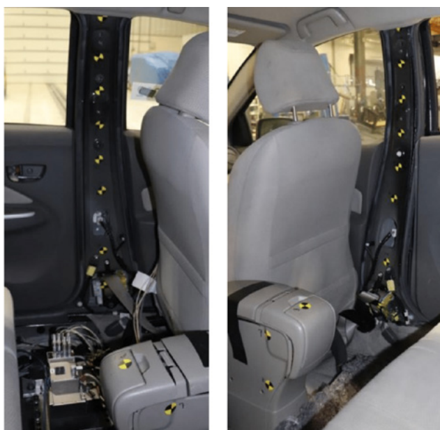
Figure 5-24 B-Pillar Deformation Measurement Locations Pre-test in Test 2
