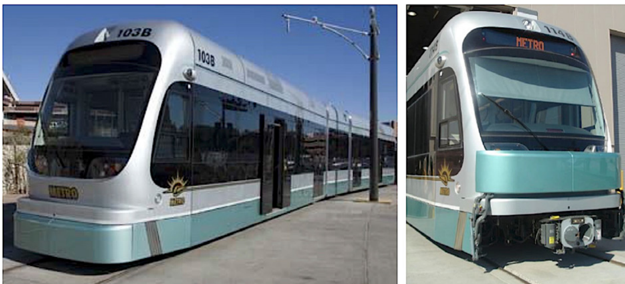
Figure 6-1 Kinkisharyo Low Floor LRV with a Front Enclosure [8]
