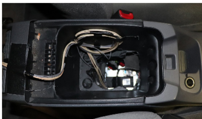
Figure 5-8 Test 1 Accelerometers Mounted at the Base of the Center Console
