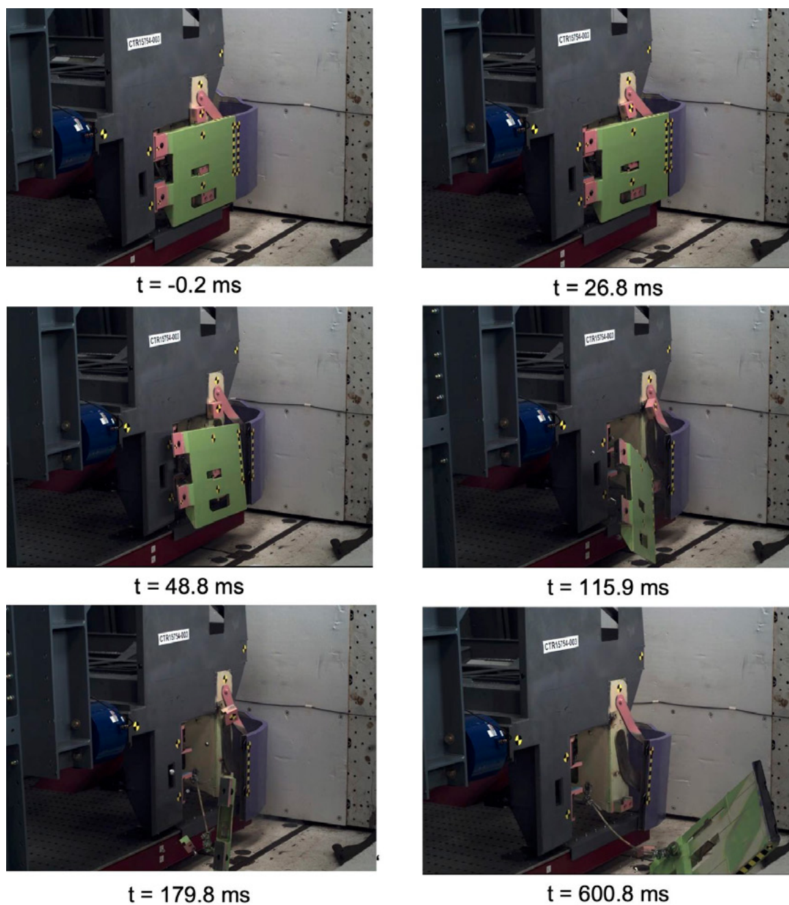
Figure 5-55 High-Speed Video (right-oblique) of Test 3
