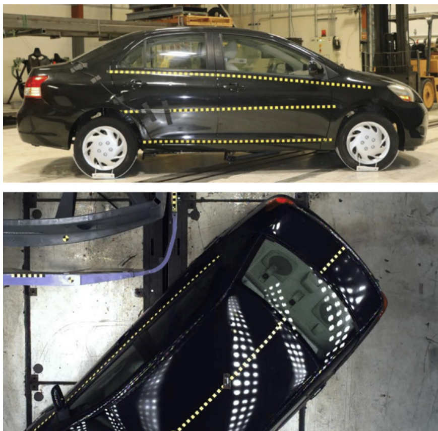
Figure 5-23 Markers on the Exterior of the 2010 Yaris in Test 2
