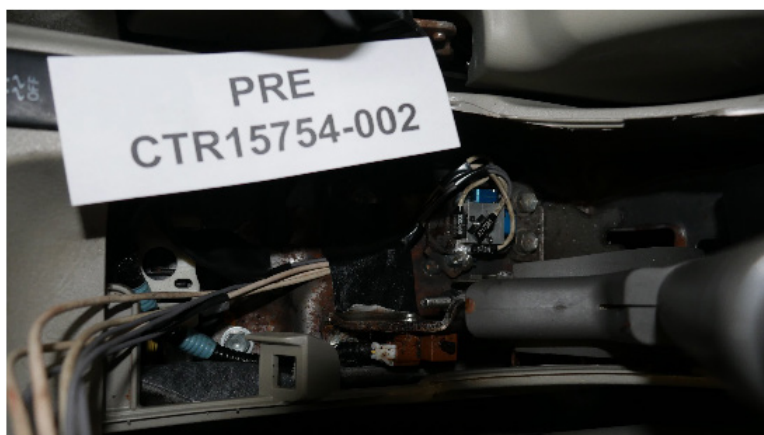
Figure 5-18 Test 2 Accelerometers Mounted at the Base of the Center Console
