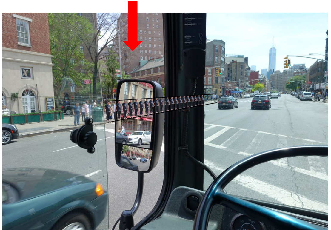
19 Pedestrians Hidden by the Pillar and Mirror
