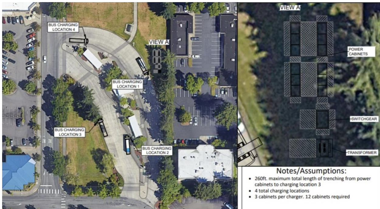
Figure 24 – Lacey Transit Center Conceptual Charging Layout
