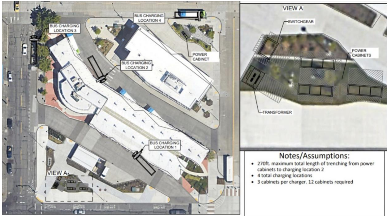
Figure 22 – Olympia Transit Center Conceptual Charging Layout
