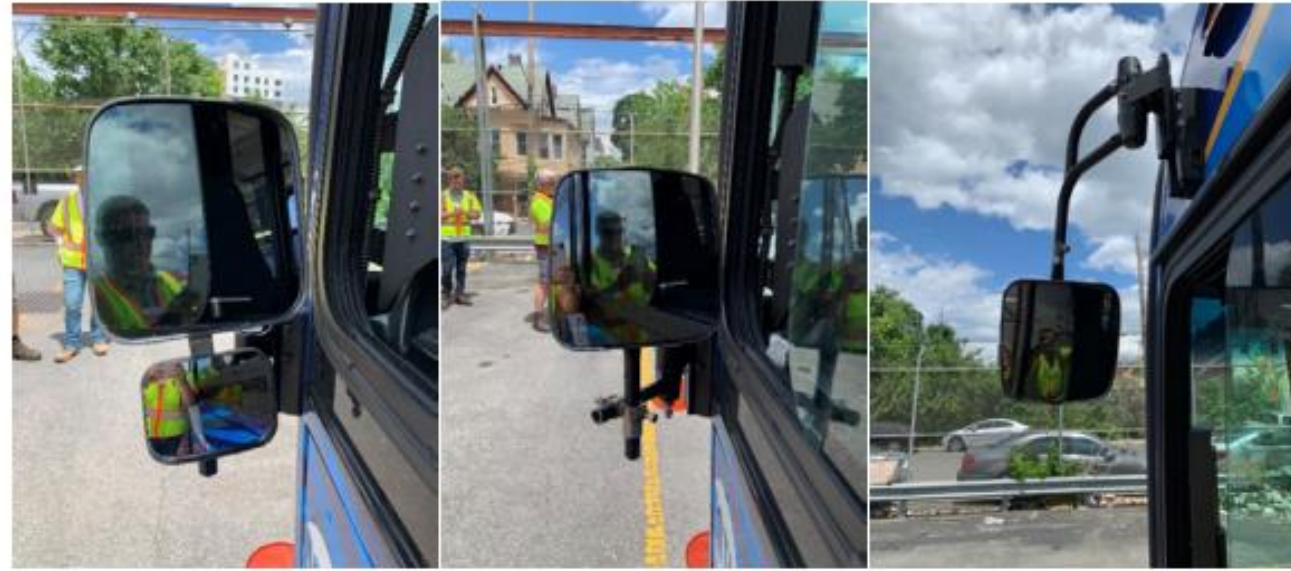
Figure 4-1 Prototype mirrors—low mount with convex (l), semi-curved low mount (c), and semi-curved high mount (r)
