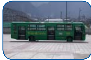
Additional doors on feeder line— Bogotá, Colombia
