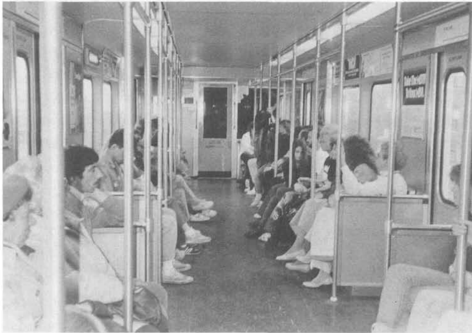
FIGURE 4-3. LONGITUDINAL ARRANGEMENT OF SEATS
