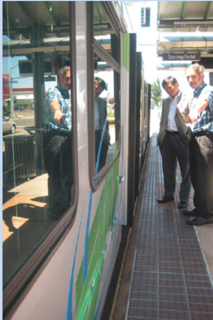
the VAA-equipped 60-ft articulated New Flyer bus and a station platform on Lane Transit District's Emerald Express (EmX) BRT route.
