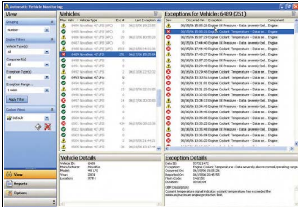
Figure 4-18: Example Vehicle Monitoring System
