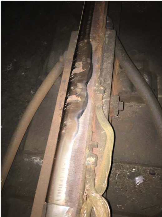
Figure 1: 1/8 th inch rail shelling at D1 098+90.
