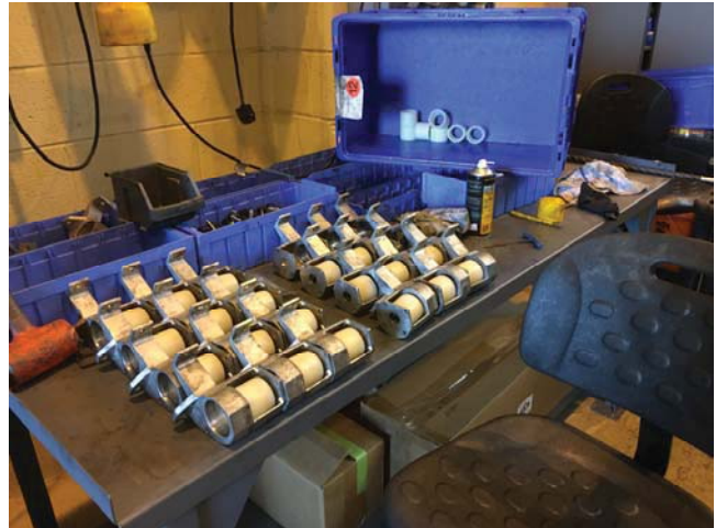
Figure 2: Contractor performing upgrade to door spindle sub assemblies
