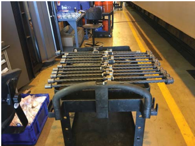
Figure 3: Rebuilt door spindles ready for installation
