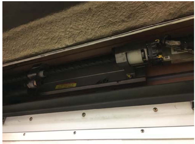
Figure 4: Rebuilt door spindle installed in rail car
