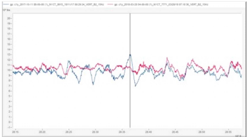
Figure 5-6 Vertical dip measured by geometry car at Woodside Station on CM track
